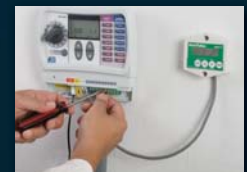
▶ Wire the SMRT-Y controller interface to the irrigation controller
