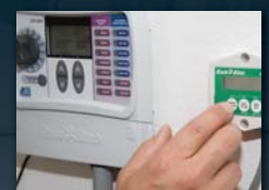
▶ Perform the auto-set function to establish the site's unique moisture threshold
